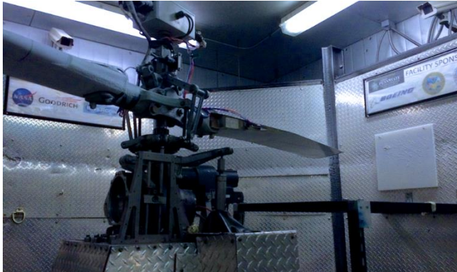
Fig. 4: Full size rotor blade mounted for anti/de-icing testing in the AERTS facility at the Penn state University in State College
