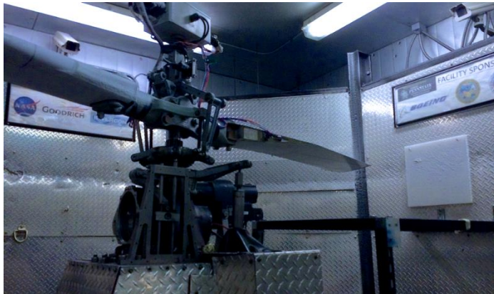
Fig. 2: Full size rotor blade mounted for anti/de-icing testing in the AERTS facility at the Penn state University in State College
